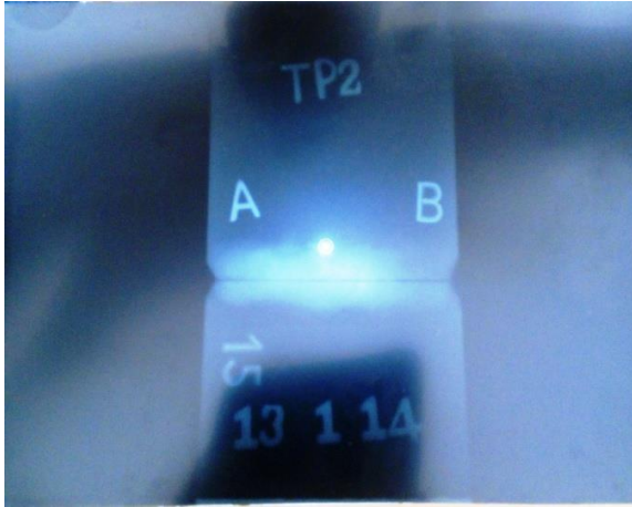
Fig 9: Radiography Test Result on Cold Crack Specimen
